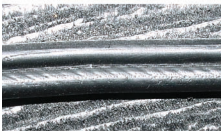
Electro-Fusion Wire on Inside of PTJC
