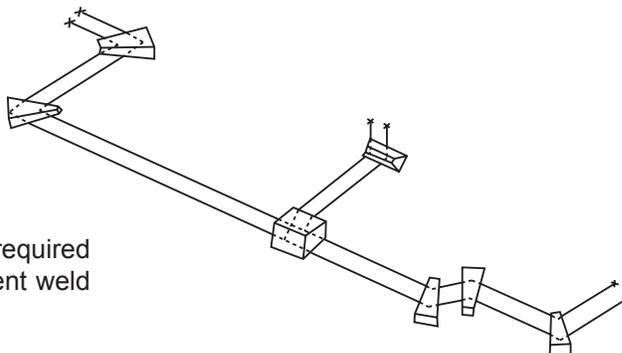
NOTE: Thrust blocks are required with gasket pipe and solvent weld fittings.
